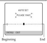
When you have connected the video recorder to a TV offering T-V Link via a fully-wired 21-pin SCART cable (Fig. pg. 11) and the TV is turned on, the recorder automatically performs the Preset Download (Fig. pg. 14) even if you select "Auto" for Auto Set Up function.
